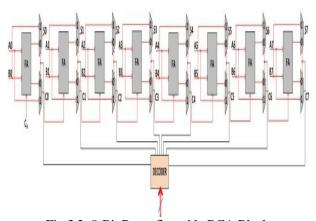
Fig 3.2: 8-Bit Reconfigurable RCA Block.
