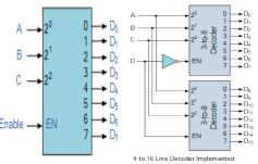
Fig 3.4: Decoder Block Diagram Decoder, Implemented with two 3-to-8 Decoder.
