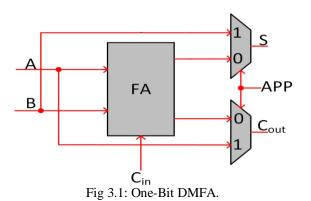
Note that the FA cell is power gated when working in the surmised mode. Amalgamation and assessment of power utilization of a 16-bit RCA were worked in Synopsys Design and Power Compiler and the relating results are depicted. Our analyses have demonstrated a unimportant distinction in the power utilization of DMFA when worked in both of the two guess modes.
